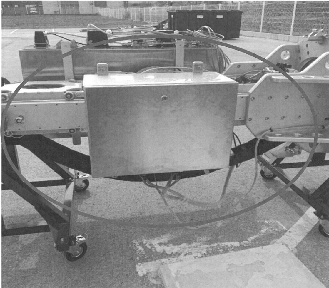
Figure 10.1. Pneumo Controller of pneumatic items
