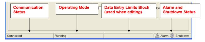
Figure 4-3. Service Tool Status Bar
