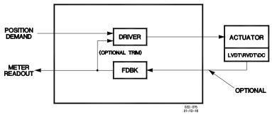
**Typical Proportional Actuator Block Diagram**
