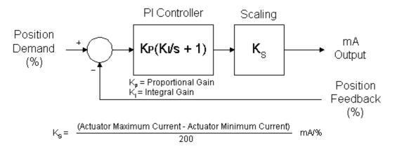
Figure 4-17. PI Control Structure
