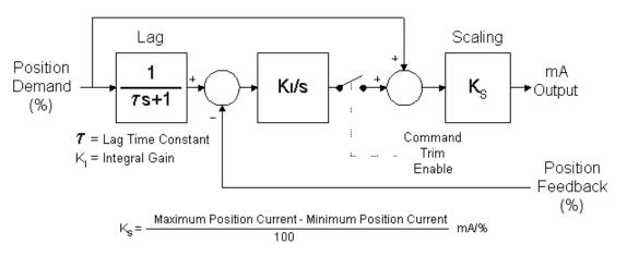
Figure 4-13. Proportional Control Structure
