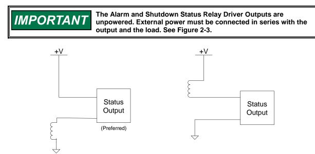
Figure 2-4. Status Relay Driver Output Wiring
