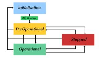
Figure D-3. CANopen Slave State Diagram
