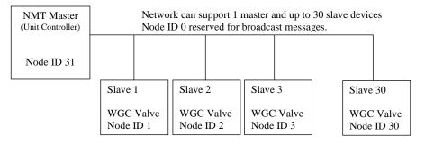
Figure D-1. Network Architecture
