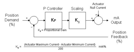
Figure 4-15. P Control Structure
