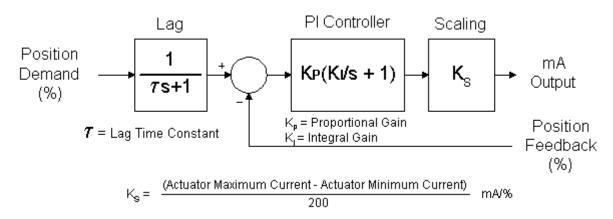
Figure 4-19. PI w/Lag Control Structure
